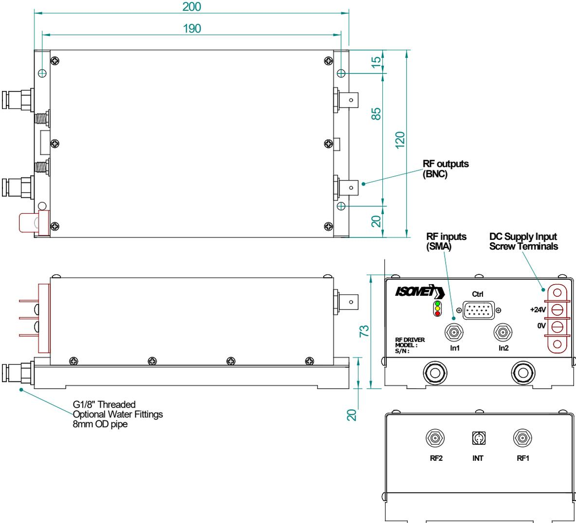
Figure 1: Driver Installation
